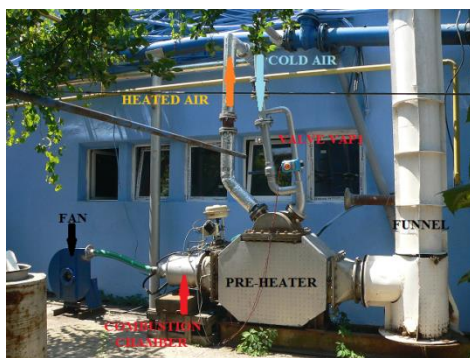
Fig. 2 a) The air pre-heater b) air preheating line diagram
