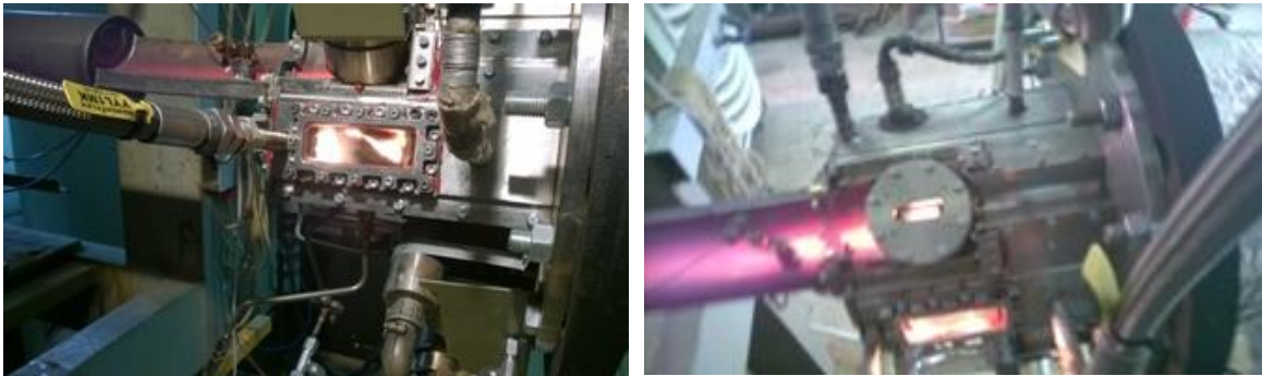
Fig. 13 Combustion chamber assembly during the tests
